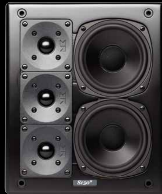
Placing the drivers side by side in close proximity reduces cabinet size significantly for enhanced structural integrity at no sacrifice in performance. Because all drivers are close to the edge of the baffle, diffraction phenomena are virtually eliminated.
