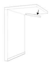
Apply again the acoustic panel on the surface and hold for 1,5 minutes and ensure it stays fixed in place.
