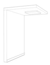
Remove the acoustic panel slightly from the wall surface (approximately 2 cm) during 15 seconds.
